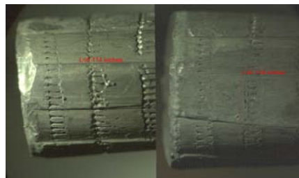
Figure 3. .38 special lead semi-wadcutter, pristine (left) vs damaged (right) groove impression
