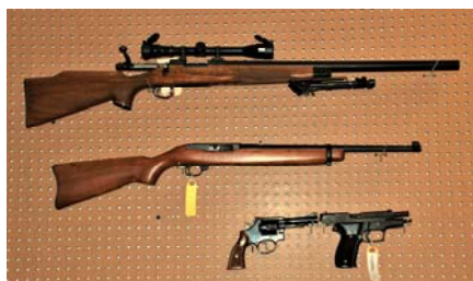
Figure 1. (from top to bottom) Remington 700 (.308 Winchester), Ruger 10/22 (.22 long rifle), Smith & Wesson Model 15-4 (.38 special), Sig Sauer P226 (9mm Luger)
